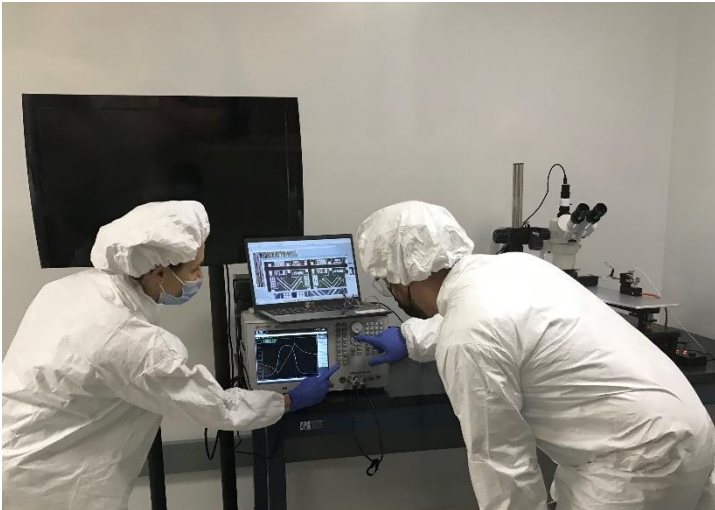
Our Class 100 cleanroom for 200 mm wafer-level test and measurement. Clients may install project-specific equipment.
